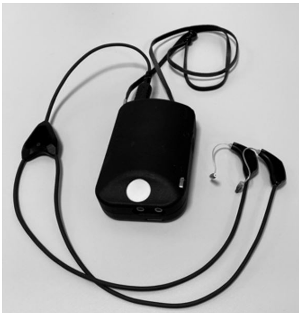
Figure 2: PHL including the processor box and wired BTE-RIC headsets; a neckband is attached to the top of the processor box.
