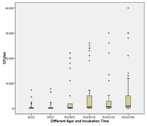
Figure 4: Aerobic heterotrophic bacteria of 36 samples from the water of distribution pipework. The boxplot diagram shows the median, interquartile range and outlier.
