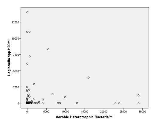
Figure 3: Scatter blot, correlating cfu of *Legionella* spp. and aerobic heterotrophic bacteria on R2A agar at 35°C after 3 days of incubation of 71 samples of output water of DCUs
