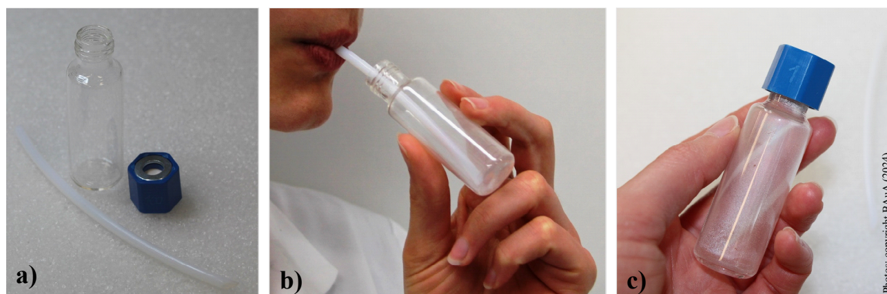
Fig. 1 Collection of an exhaled-air sample: a) 20-ml screw-top glass vial, assembled open-top screw cap with PTFE-lined septum, and PTFE tube, b) specimen collection, and c) sealed, gastight 20-ml screw-top glass vial containing the exhaled-air sample
